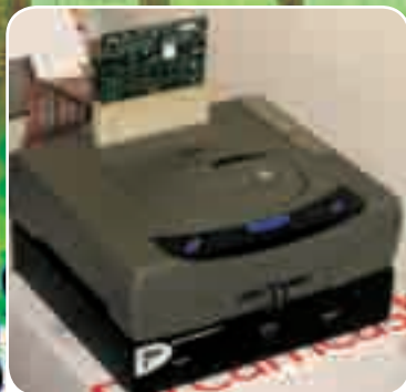
» A Saturn development setup. Notice the custom chip board in the back, and also the large development box underneath. Essential for running certain pieces of code.
